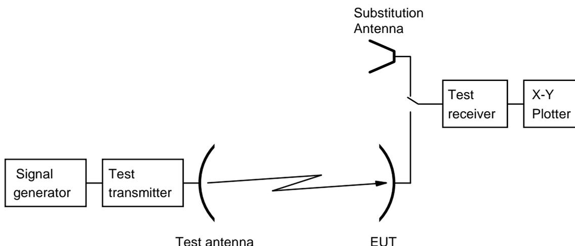
**Figure 6: Test arrangement - antenna transmit gain measurement**
