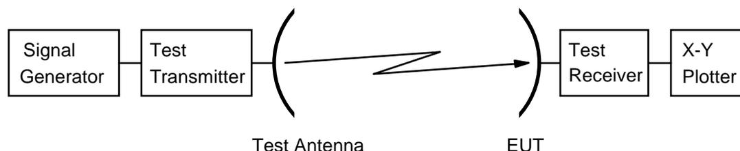
**Figure 8: Test arrangement - antenna receive pattern measurement**
